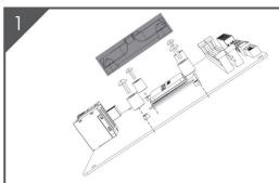
Remove the radiator bracket that comes with the AMD motherboard, keep the screws and the original AMD backplate, and then insert the AMD-specific limit post into the backplate nut.
