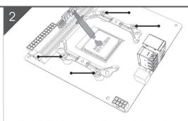
According to the direction shown in the picture, use the 4 screws that come with the AMD bracket to lock the buckle on the backplate, and then evenly apply a layer of thermal conductive silicone grease on the surface of the CPU.
