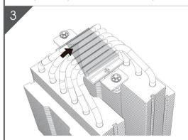
Take the fans off the heatsink and peel off the protective film on the bottom
