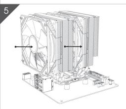
Install the fan on the heat sink, paying attention to the airflow direction. Plug the heatsink power connector into the CPU Fan pin on the motherboard.
