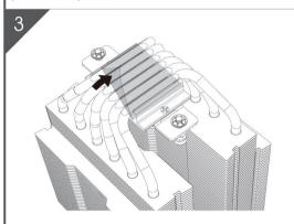
Take the fans off the heatsink and peel off the protective film on the bottom of the heatsink.
