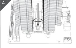
Place the heat sink on the mounting bracket and align the holes of mounting bracket, then use a screwdriver to lock the radiator to the mounting bracket.
