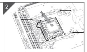
According to the direction shown in the figure, use 4 Intel-specific screws to lock the buckle on the backboard, and then evenly apply a layer of thermal conductive silicone grease on the surface of the CPU.
