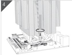
Place the heat sink on the mounting bracket and align the holes of mounting bracket, then use a screwdriver to lock the radiator to the mounting bracket.
